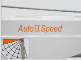
Auto II Speed automatically reduces the maximum working speed of all crane functions when a load is sensed.
