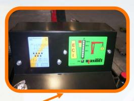
Console with receiver and electronic capacity indicator (ECI)
